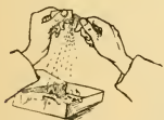
Striking fire with flint and steel. The sparks were caught on some old, half-burnt rag, and were then blown to a blaze.
